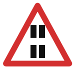
Gap in median
